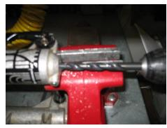
12.On the Damper leg, drill with a 10 mm drill slowly blowing off the
