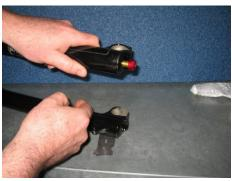
24. Thread the nut with the o-ring facing the lower leg
