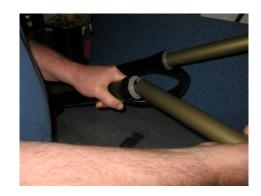
16. Grease the oil and dust seal with your choice of grease and re-assemble the slider tubes to the lower casting
