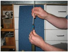
**27.** Cycle rod to remove any air bubbles and insert the rebound adjust rod. Fully compress the rod and stanchion tube.
