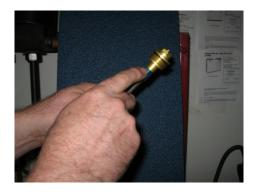
29. Screw on the fork cap. Make sure rod bottoms out before the jam nut!
