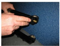
22. Push it thru until the ABS cone bottoms on the lower leg
