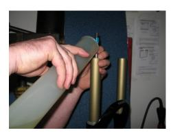
**26.** Pour oil into upper leg allowing oil to settle into the cartridge, pull the rod and stanchion tube up and down a bit until it is filled about an 55 mm from the top fully compressed, Lyrick stanchion not shown.
