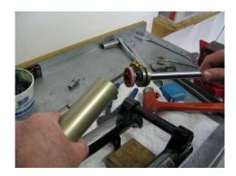
9. Insert a coat hanger or welding rod with a slight hook at the end and remove the stock rubber bottom out bumper (discard, this it will not be used)
