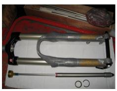
17. Prepare to install the Damping Cartridge
