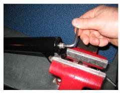
4. Using a 5 mm Allen key loosen the bolt 4-5 turns
