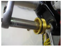
18. First Remove the Remove the Fork Cap with a ½ open
