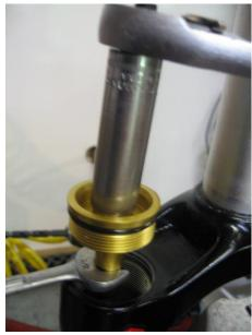
**30.** Bring the jam nut up to the fork cap and tighten with a slight squeeze on the two wrenches, approximately 10 in-lbs, be careful not to over tighten as , Totem shown, Lyrik similar.
