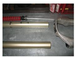
8. Remove the snap ring and rebound damper rod assembly
