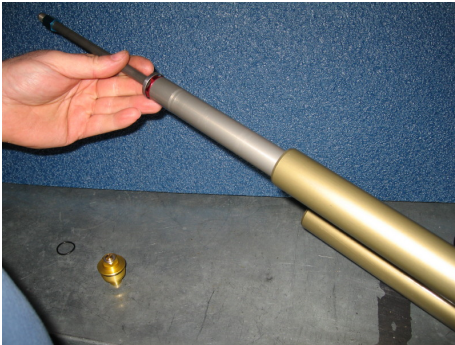
Guide the cartridge assembly thru the entire slider tube
