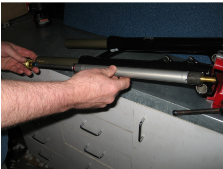
Lightly torque the cartridge tube cap, tube and compression bolt as one, do not over tighten as it will deform the cartridge tube.
