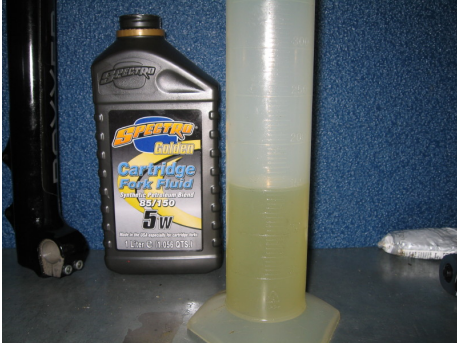
Measure out 150 cc (standard amount) of cartridge fork oil 85/150
