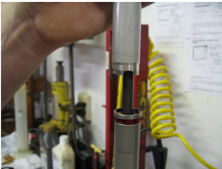
Slip the cartridge cap removal tool over the cartridge rod
