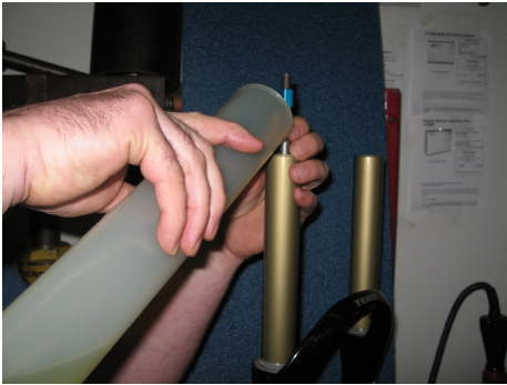
Pour oil into upper leg being careful not to spill any
