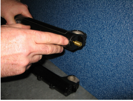
Push it thru until the ABS cone bottoms on the lower leg
