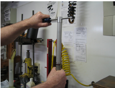
Apply torque to loosen the compression bolt adaptor
