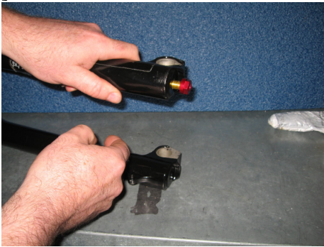
Thread the nut with the o-ring facing the lower leg
