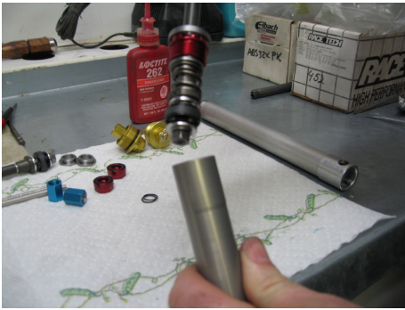
Remove cartridge rod assembly from cartridge tube
