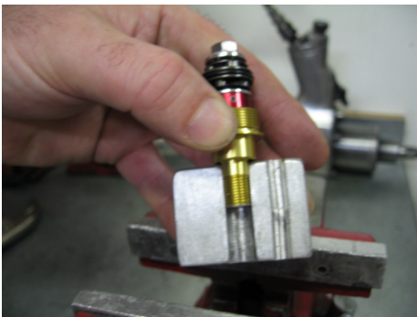
Insert the compression bolt assembly into the 10 mm shaft clamps
