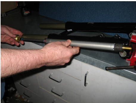
Prepare the cartridge kit as shown, remove the fork cap
