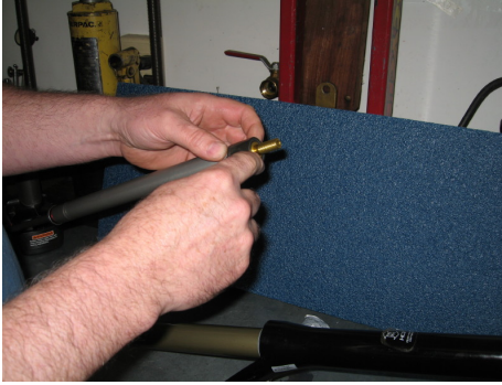
Inset the o-ring into the bottom groove
