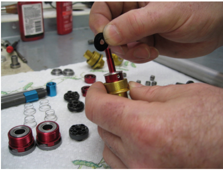
Remove compression valving shims and set aside for revalving
