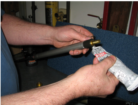
Use RTV to help secure the -018 o-ring to the bottom of the ABS cone
