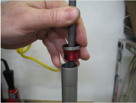
Remove the cartridge tube cap
