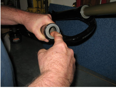
Grease the oil and dust seals with your favorite slippery grease
