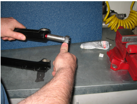
Tighten the nut to 10-15 in-lbs
