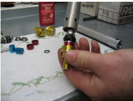
Remove the compression bolt adaptor assembly
