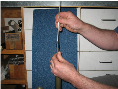
Cycle rod to remove any air bubbles and insert the rebound adjust rod
