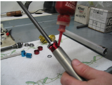
Apply a drop of red loctite to the threads
