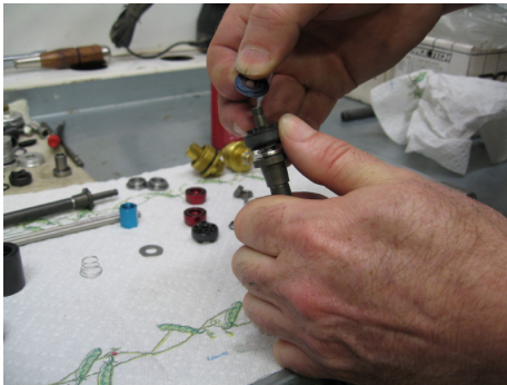
Remove the shim stack and set aside for revalving
