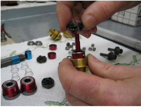
Remove compression piston valve
