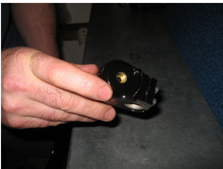
Line the 10 mm adaptor bolt to the lower hole
