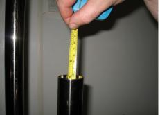
After all air bubbles are removed and damping is smooth through out the stroke. Measure down to the top of the compressed stanchion to the oil, standard is 125 mm for the Boxxer 32, and 55 mm for the Totem and the Lyrik. Using a suction tool or just dump oil out until desired height is reached
