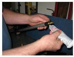
Use RTV to help secure the -018 o-ring to the bottom of the ABS cone
