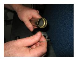
Remove all the components so the slider bottom hole is empty
