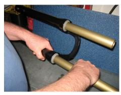
Push the slider tube all the way in until it contacts the bottom of the leg
