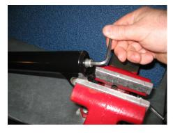
Using a 4.5 mm allen key loosen the bolt 4-5 turns
