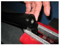
Deburr the hole and remove any visible chips
