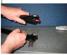
Thread the nut with the o-ring facing the lower leg
