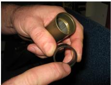
The oil lock ring will have an arrow pointing to the champher, this will face out or down to prevent damage when sliding over the ABS cone.
