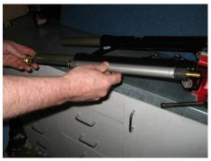
Prepare the cartridge kit as shown, remove the fork cap
