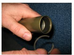
Insert the oil lock ring (ABS insert) with the internal chamfer facing out
