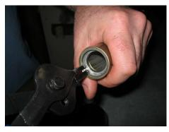
Using snap ring pliers remove the ring from the bottom of the slider leg
