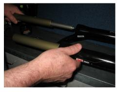
Pull the slider tube and damper rod from lower legs
