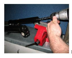
Drill with a 10 mm drill slowly blowing off the chips to avoid falling in
