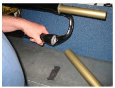
Reinsert the slider tube in the lower leg
