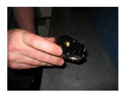
Line the 10 mm adaptor bolt to the lower hole
