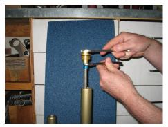
Bring the jam nut up to the fork cap and tighten with a slight squeeze on the two wrenches, approximately 10 in-lbs, be careful not to over tighten as theses parts can easily be damaged
