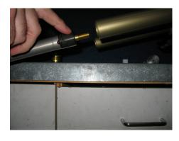
Insert the cartridge assembly into the slider/lower leg, take care to not knock off the base o-ring
