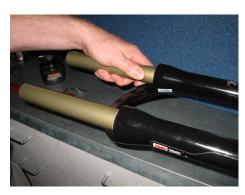
Remove the slider tube being careful that the chips remain in the tube
