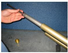
Guide the cartridge assembly thru the entire slider tube
