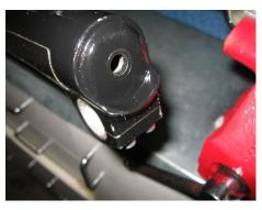
This end of the lower leg will need the internal 10 mm hole extended thru
