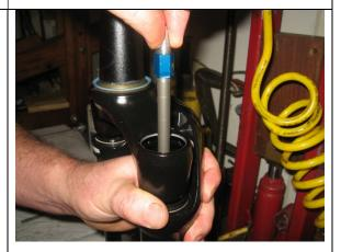
Cup your hand over the top and use it to pressurize the leg as you compress the stanchions to help remove the air bubbles, if needed assemble the fork cap temporarily to help this process maybe easier.
