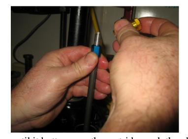
Attach the fork cap by screwing cap on until it bottoms on the cartridge rod, then bring the blue jam nut up to secure it to
