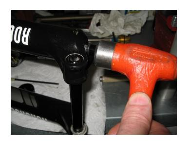
Tap the loosened bolt to relieve the lower press fit.
