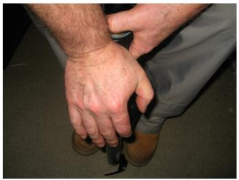
Cup your hand over the top and use it to pressurize the leg as you compress the stanchions to help remove the air bubbles, if needed assemble the fork cap temporarily to help this process.
