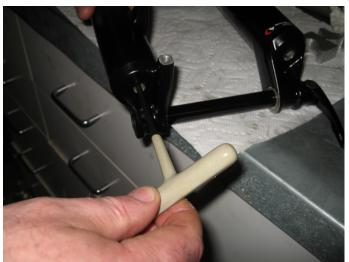
Use either the 100 mm bolt or a thandle Allen to press the air shaft past the lower seal to relieve the negative spring pressure. The 100 mm bolt makes it easier to pull the air shaft back out, if you do not have this bolt use a Philips screw driver to center the air shaft as you pull it back out.
