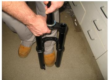
Remove air side fork cap and try to equalize the negative air chamber by pulling up and holding until the negative spring pressure is released, generally this is difficult to do, so we will step you through the air shaft equalizing method. The fork needs to be fully compressed to install the cartridge, this is also a good thing to do regularly to keep the negative spring pressure from building up.
