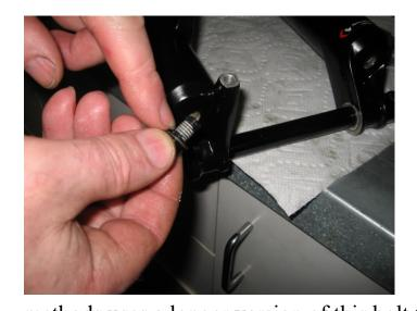
The bolt is a M8 x 1.25, one of the two methods uses a longer version of this bolt to help equalize the negative spring. You
