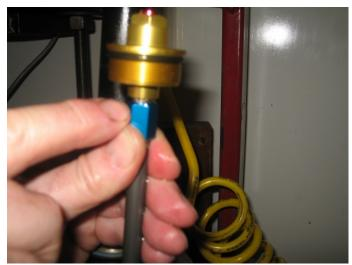
Thread the fork cap on fully to the grey
