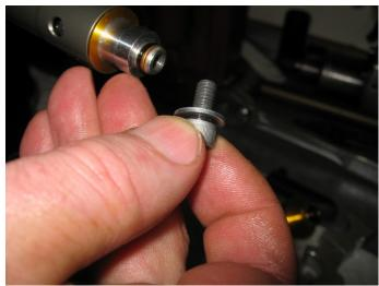
Remove the 6 mm socket head cap screw and washer from bottom end of cartridge and set aside.
