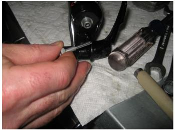
Use the small fat bladed tool to adjust the compression, 22 click full clockwise is the firmest setting, softest is all the way counterclockwise. Standard is 11 clicks out. from full hard. Diameter is .132 inches and the blade is .060 thick.
