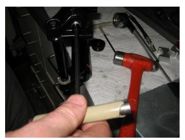
Reinstall the lower bolt, torque to
