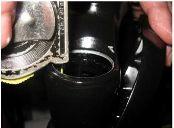
Measure from top of stanchion down to oil with the fork fully compressed and the cartridge rod pressed all the way down. The height of oil needs to be 35 mm from the top. Over fill will cause fork seal damage, under filling will cause the cartridge to suck air and have erratic damping.
