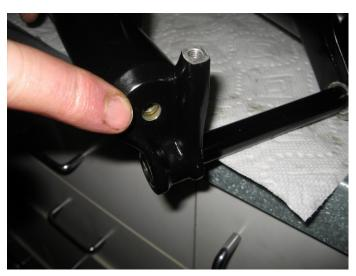
Reinstall the air side fork cap. Torque per Rockshox specs.
