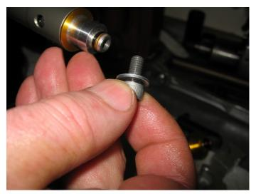
Remove the 6 mm socket head cap
