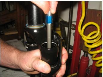
and cycling the stanchions up and down until the level stops dropping.
