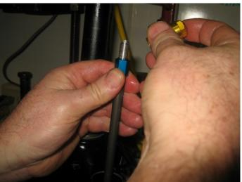
Attach the fork cap by screwing cap on until it bottoms on the cartridge rod, then bring the blue jam nut up to secure it to the rod.
