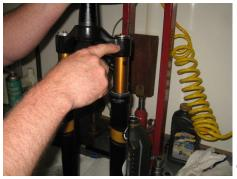
Thread the fork cap in by hand initially
