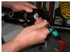
Depress the Shrader valve with a screwdriver to release the air pressure Skip this Step if your fork has a mechanical spring
