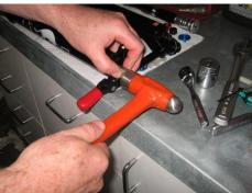
Tap the nut with a soft face hammer to un-seat the press fit. Do not strike the lead of any exposed external thread. It will damage it!
