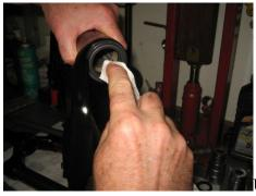
Using a clean paper towel wipe off any old grease and dirt from the dust seal
