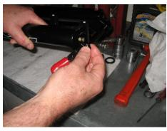
Slide the factory washer onto the air or spring shaft
