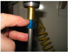
Thread the fork cap on fully to the grey shaft until the threads bottom out.
