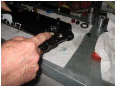
Push the assembly together and the air spring shaft should go through the casting. A small screw driver can be helpful to gently align the shaft to the hole.
