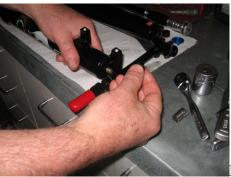
Remove the spring retaining nut and seal washer
