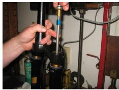
Cycle the damper rode up and down until the oil has no air bubbles visible
