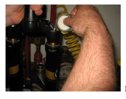
Measure the oil height makes sure it is 35mm(standard) from the top of the fork repeat the previous step until the correct reading is achieved
