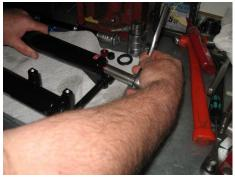
Tighten the retaining nut, be careful not to over tighten as they are small aluminum parts, typical torque is 15 inch-lbs
