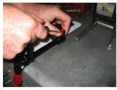
With an Allen key, remove the low speed knob.
