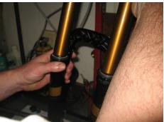
Gently reassemble the fork sliders to the lower casting. Don't force this step. It helps to get one seal started first then rock it over to the second. After both seals have accepted the sliders gently slip the tubes past the bushings.
