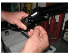
Remove the small spring from the compression knob assembly
