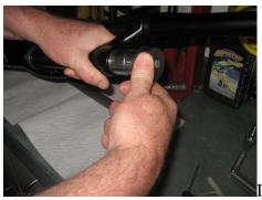
Loosen the for cap using a 28 mm 6 point ratchet
