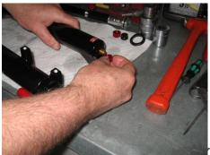
Thread the red retaining nut with included O-ring onto the assembly
