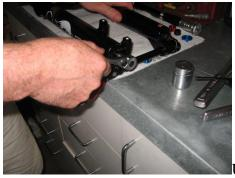
Using a 10mm Ratchet loosing the retaining nut on the spring leg
