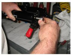
Tighten the nut snug, do not try to torque as it will just crush the washer
