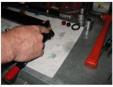
Thread the factory nut onto the shaft
