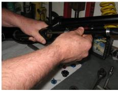
The fox F.I.T cartridge should slide out of the fork easily
