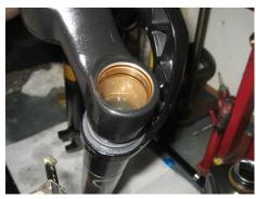
Fill the Damper tube with 85/150 oil to near the top as shown
