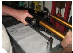
Gently separate the upper sliders from the lower casting
