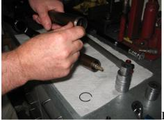
Install the abs oil lock ring, with the I.D. champher facing out.
