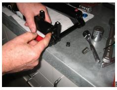
Push the sprung rod through the casting
