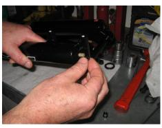
Push the gold end through the fork casting as shown. Use a small screw driver to help line up the assembly
