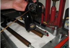
Remove the bottom out bumper you will not need this, only on the damper side, the air side bumper can remain installed to prevent damage to the stanchions from severe bottom out.
