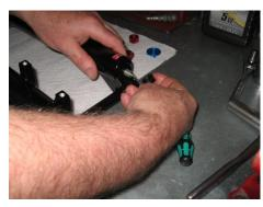
Remove the retaining nut fully
