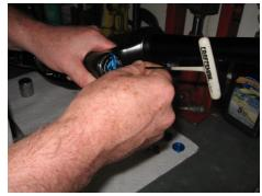
Using a 2mm Allen wrench loosen remove the bolt retaining the compression knob
