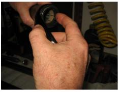
Apply new grease to the dust seal
