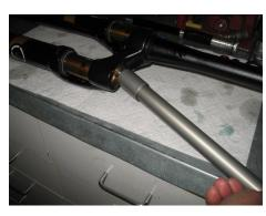
Insert the Avalanche Cartridge into the damping leg
