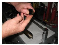
Insert the retaining ring back into the groove. Make sure it is fully seated before proceeding to the next step.
