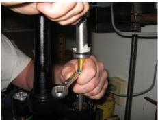
Using a ½ inch wrench and 15mm 6 point socket tighten the jam nut. **Be**
