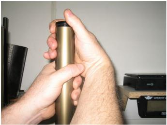
Hand tighten the outer fork cap.
