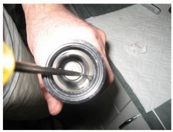
The larger of the two steps is the fill line for the cartridge
