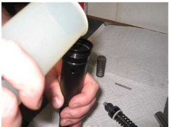
Pour oil approximately 5 mm above the fill line, cycle the cartridge rod a few times to bleed the rebound circuit and recheck the oil level, add as necessary to maintain this oil level.
