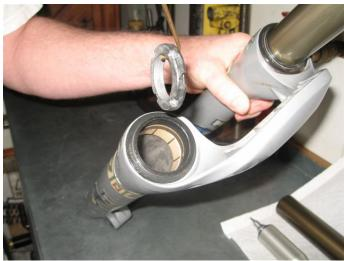
Remove the bottom out bumper with a coat hanger or welding rod.
