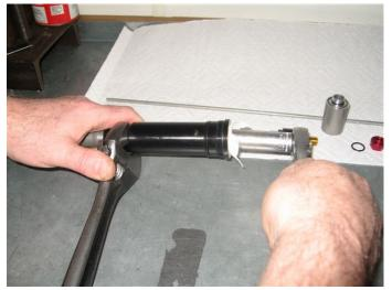
socket loosen the inner fork chamber cap assembly.
