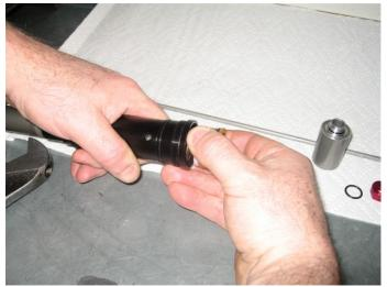
Remove the inner chamber cap assembly.
