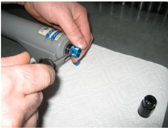
With an Allen key, remove the high speed knob.
