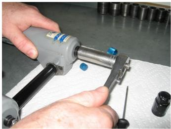
Remove base bolt adjuster nut.
