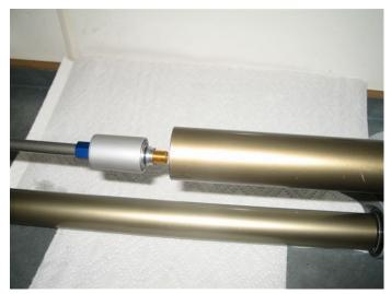
Remove the cartridge damper assembly.
