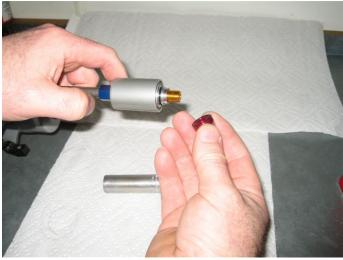
Remove the red nut and o-ring.
