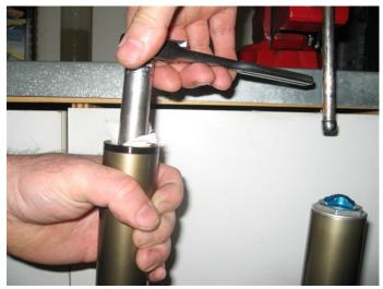
With a 15 mm 6 point socket remove the outer chamber
