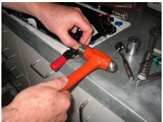
On the Sprung side tap the nut with a soft face hammer to un-seat the press fit. Push the spring assembly though the casting just like the damper side. **Do not strike the lead of any exposed external thread. It will damage it!**
