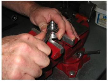
torque, after bottoming tighten 1/16 turn.
