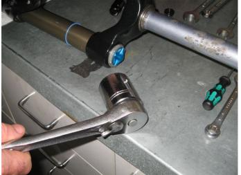
Remove fork spring/air cap to allow fork s to be
