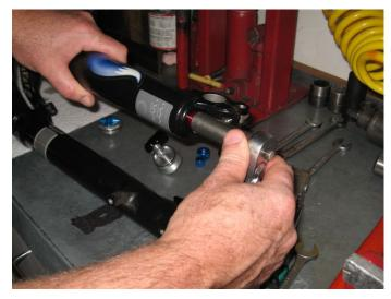
Snug up adaptor nut and tighten to 15-20 inch-lbs.
