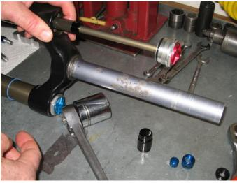
Be careful when removing, their maybe excess oil that needs to be dumped. Leave the bottom-out bumper in, if needed remove it for cleaning lower casting internals.
