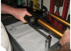
Gently separate the upper sliders from the lower casting
