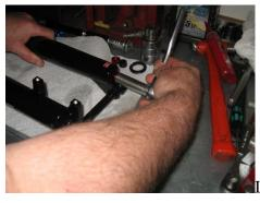
Loosen the retaining Nut on the Sprung side of the fork
