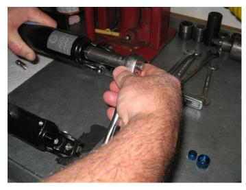
Loosen base nit with 15 mm socket.
