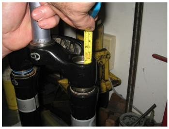
For 2006-14 models, adjust oil height to 30 mm(1.18 inches) from top with all components fully compressed. For 2015-17 models, adjust oil height to 40 mm(1.57) inches) from top with all components fully compressed.
