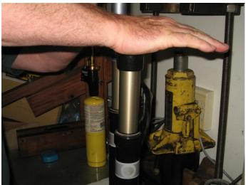
Pressurize the stanchion by placing palm of hand over
