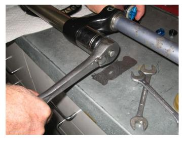
Install fork cap and tighten per Fox manual.
