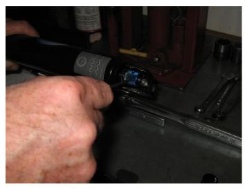
Remove high speed knob set screw and knob.
