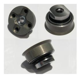
SSD valve set-up with high speed shim stack based on linkage and rider ability
