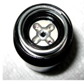
SSD valve installed in place of Boost valve
