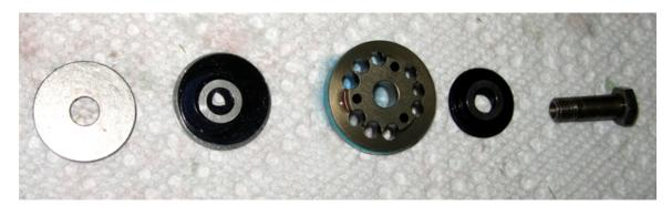
Compression revalved to rider style/speed and linkage Rebound revalved to rider weight(spring rate) and type of riding main piston and piston bolt remain unchanged
