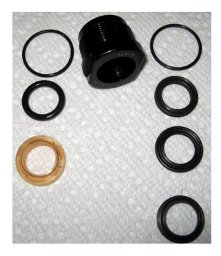
Seal head rebuilt with low friction triple sealed system
