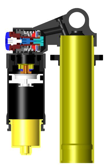
Transition Adjuster and SSD valve shown installed
