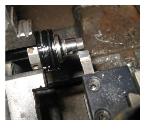
Modify High Speed arbor to accommodate Transition Adjuster piston
