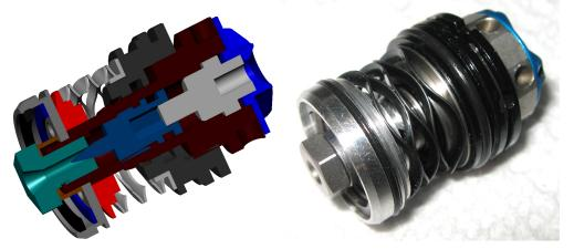
Low Speed Plunger and High Speed Valve
