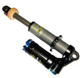
Fox RC4 with SSD, Transition and Shape Factor Bottom-out Bumper upgrade.
