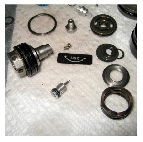
Disassemble High/Low speed adjuster
