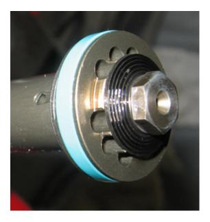
Main Piston shown with revalved shims installed
