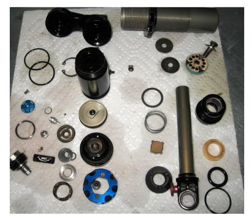
The RC4 is completely disassembled
