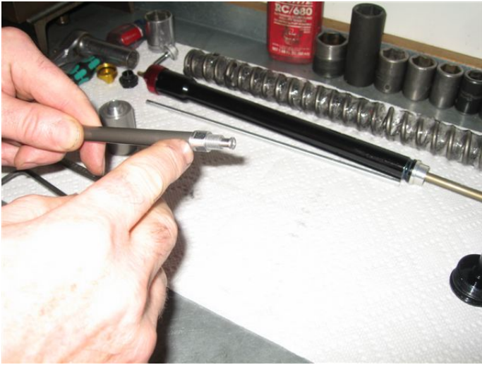
Install jam nut with round end on first.
