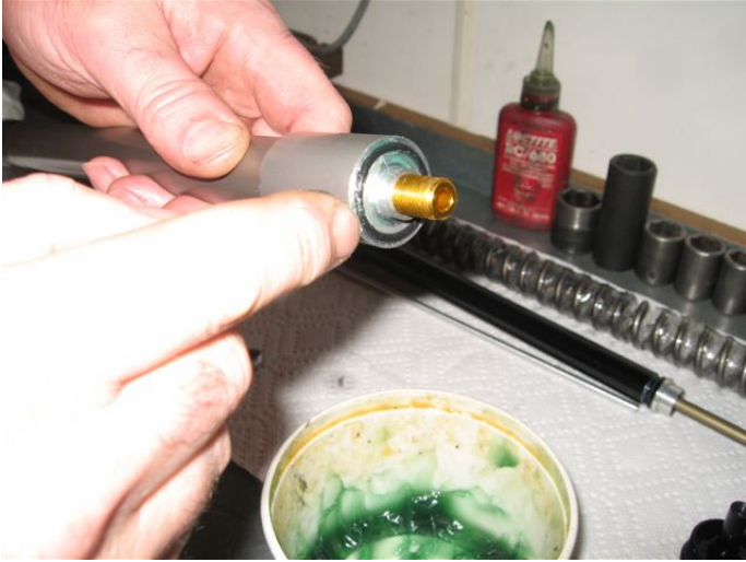
Install o-ring (20 x 2.0)
