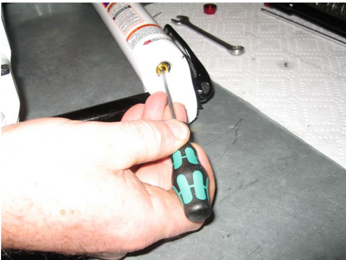
Use the allen driver to help center it through the hole.
