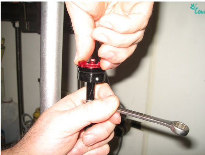
Make sure the rebound adjuster move freely.
