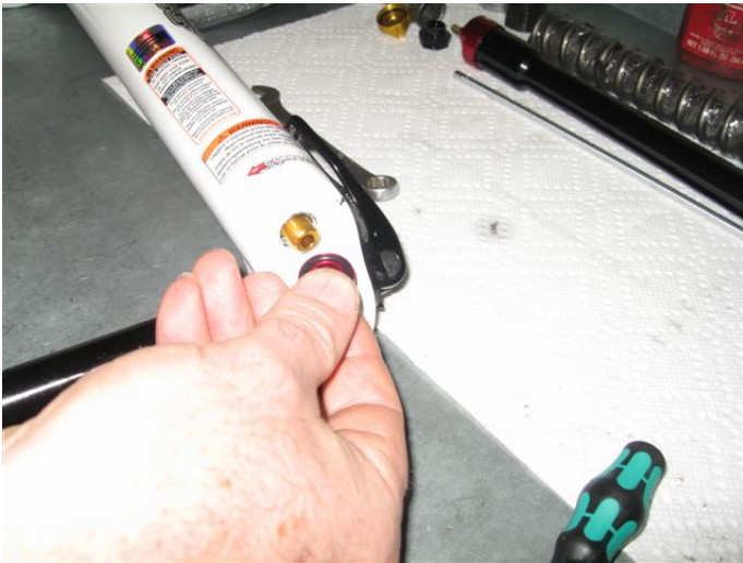
Install the nut and o-ring (-014)
