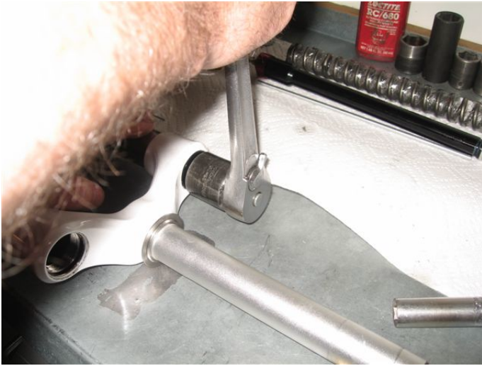
Torque to Marzocchi specs.
