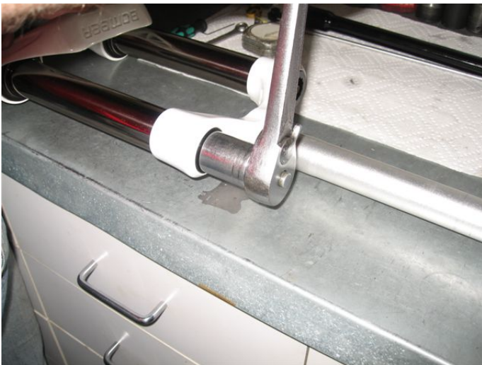
Torque to Marzocchi specs.
