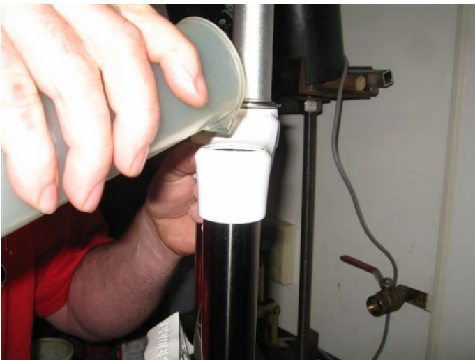
Add 50 cc of fork oil to the spring side.
