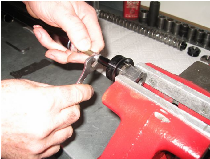
Remove the fork rebound cap from the damper rod, using a 10 mm wrench and the cassette socket.
