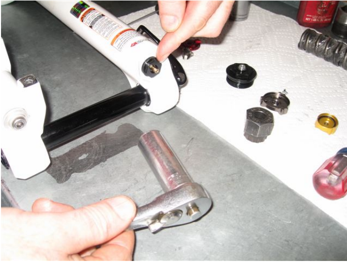
Remove base nut with 17 mm socket
