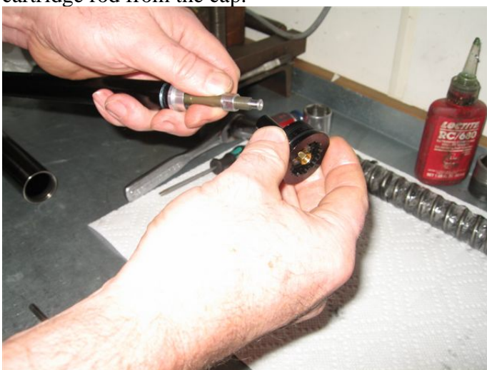
Loosen the jam nut and use it to continue loosening the cartridge rod from the cap.
