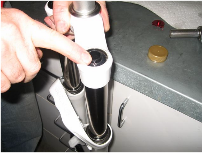
Install the upper plastic spring collar.
