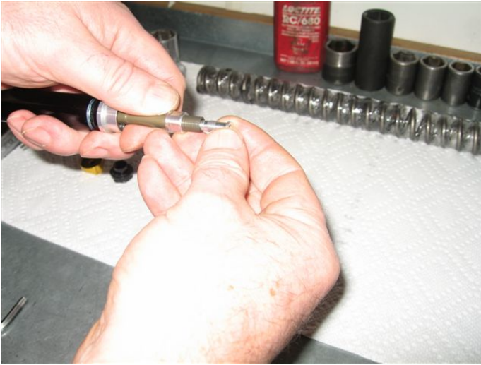
Unscrew the rebound adjuster rod from the cartridge rod.
