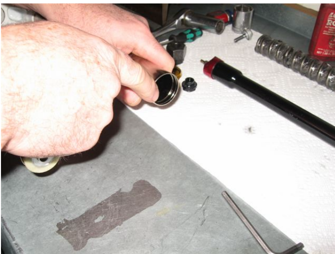
Inspect lower stanchion for damage or debris.
