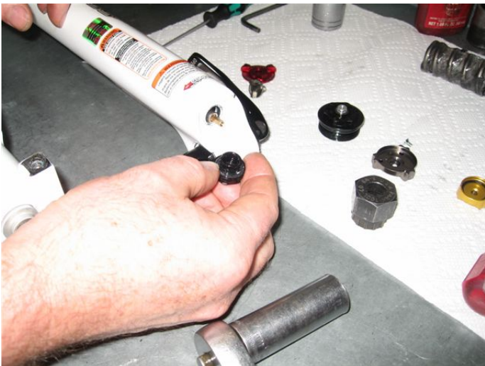
Tension the fork to help keep the internals from spinning when removing the nut.
