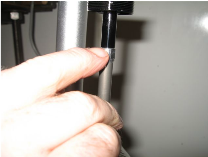
It should bottom on rod before contacting the jam nut.
