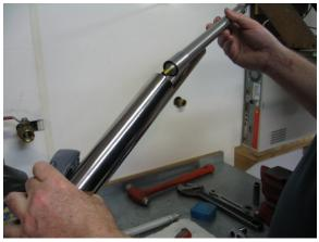
Install the cartridge in the lowers, be sure the o-ring provided does not fall off, you can use grease or rtv to help secure it.
