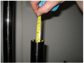
With the stanchion and cartridge rod fully compressed adjust the oil height to the value given in the set-up cart of your invoice. Range 110-140 mm.
