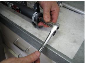
tighten to approximately 15-20 inch-lbs. It maybe necessary to use an impact wrench at the lightest setting to keep the internals from spinning and cinch-up the nut securely.
