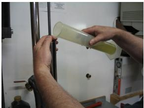
Poor approximately 300 ml of cartridge fork fluid into the damper leg, cycle the rod and stanchion up and down until all the air bubbles have dissipated.
