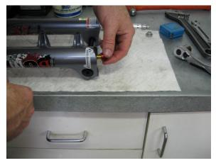
Install the o-ring and base nut.
