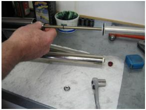
Pull the damper and spring assembly from the upper slider tube, it will take a good deal of pulling to overcome the o-ring friction to remove it Dump any remaining oil from the damper and lower casting
