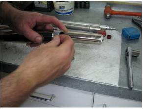
Install the oil lock ring with the inside chamfer facing out/down,
