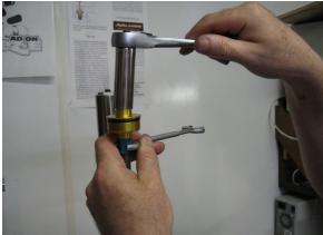
Install fork cap, be sure that the cap bottoms on rod and bring thje blue jam nut up to the cap and tighten them together, approximately 1-2 foot-lbs, be careful not to over tighten as the parts will fail if over torqued.
