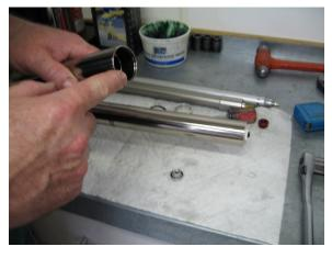
Locate and inspect the lower grooves in the stanchion.
