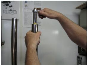
Fully extend the stanchion and cartridge rod before screwing the fork cap on. The cap does not need to be torqued, snug is sufficient as the upper crown will pinch it securely when installed.
