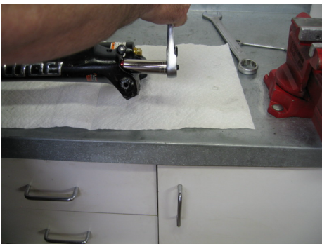
Tighten the adaptor nut to 10-15 inch-lbs
