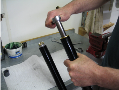
Tighten fork cap snugly
