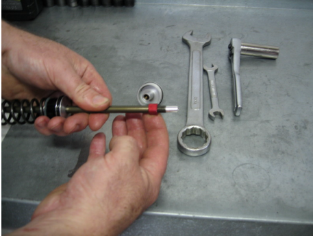
Remove the jam nut
