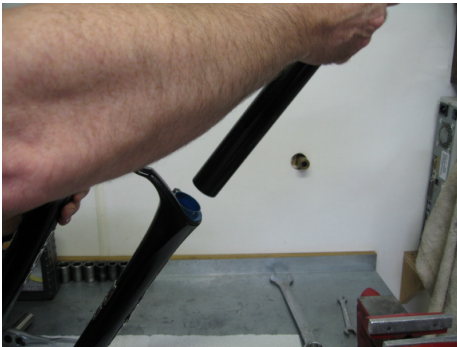
Clean and grease the seals before assembling the slider tube
