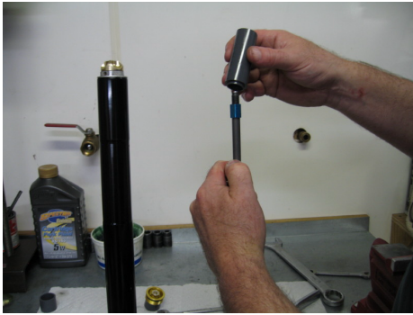
While holding the rod install the spring spacer, small end down
