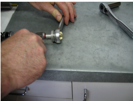
Loosen the fork cap from the damper rod and jam nut
