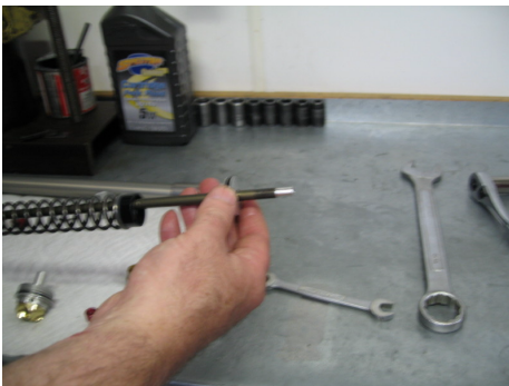
Remove the spring retainer
