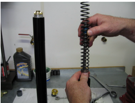
Install the spring perch with the small side down, pull the rod all the way up
