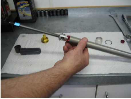
It should fit snugly over the insert o-ring on the end of the cartridge cap
