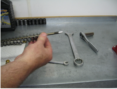
Remove the spring centering plastic washer and spring
