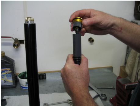
Install the fork cap and upper preload spacer
