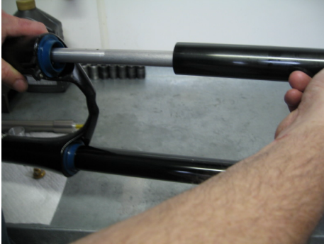
Pull the slider tube and damper rod from lower legs
