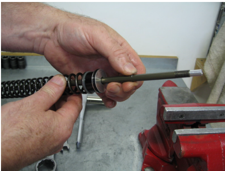
Remove the clip by sliding it off the rod
