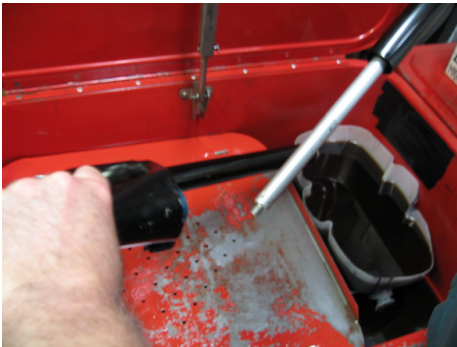
Dump any remaining oil from the damper and lower casting
