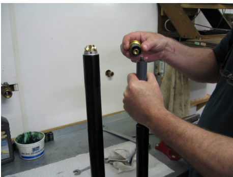
Remove the preload spacers
