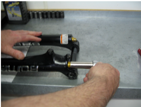
Using a 15 mm socket loosen the base nut of the Compression leg
