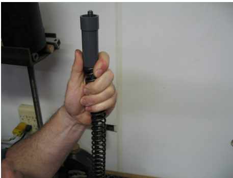
Install the spring over the rod, if your fork is 2005 and older the springs will be 306 mm long, for 2006 and newer the spring will be 340 mm long
