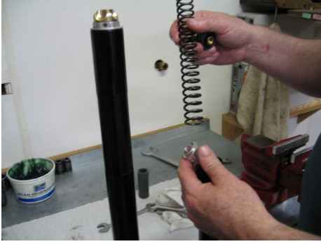
Remove the spring and spring perch
