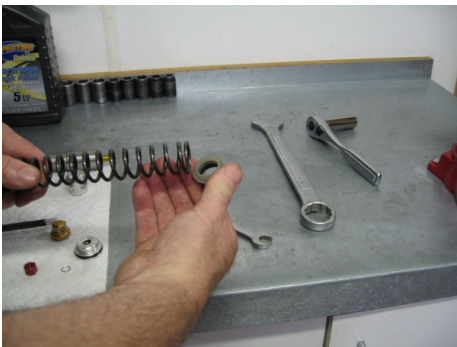
Remove the spring spacer caps
