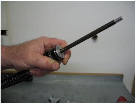
Pull back the spring retainer cap to expose the clip grooves
