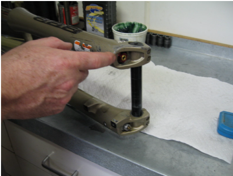
Tighten by hand to make sure the o-ring seats cleanly
