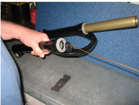
Remove the bottom out bumper and discard, this will not be used
