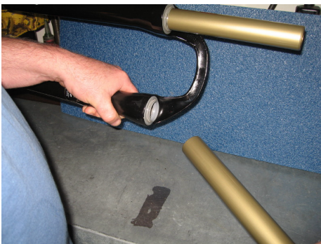
For the 32mm Boxxer reinsert the slider tube in the lower leg
