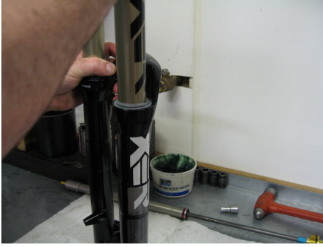
Insert the slider tube shown in the 35 mm Boxxer
