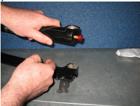
Thread the nut with the o-ring facing the lower leg
