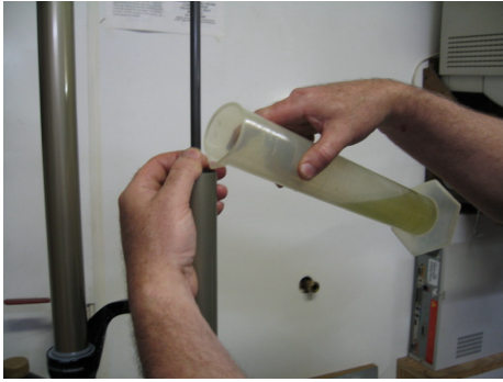
Pour oil into upper leg being careful not to spill any shown in Boxxer 35
