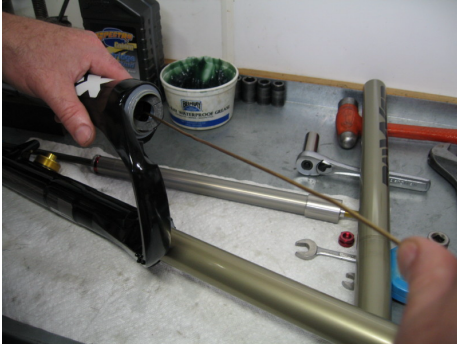
For the 35 mm Boxxer the bottom out bumper shown being removed
