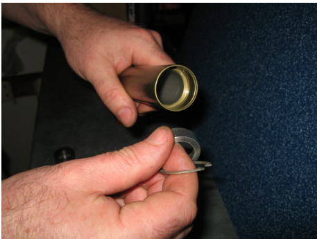
For the 32mm Boxxer using snap ring pliers remove the ring from the bottom of the slider leg
