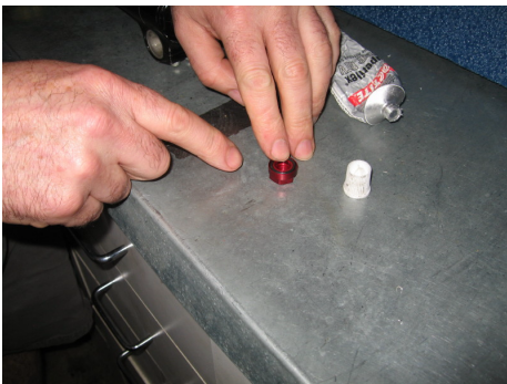
Prepare the 10 mm adaptor nut with RTV to help secure the -014 o-ring
