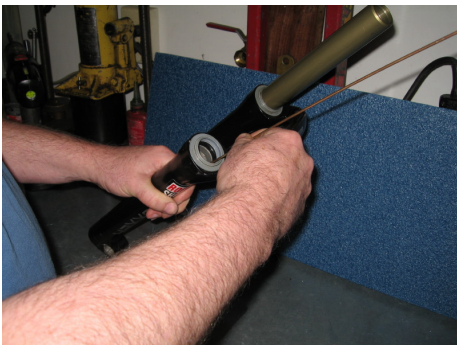
Reach to the bottom of the lower leg and hook the bottom out bumper
