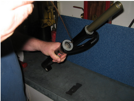
Insert a coat hanger or welding rod with a slight hook at the end
