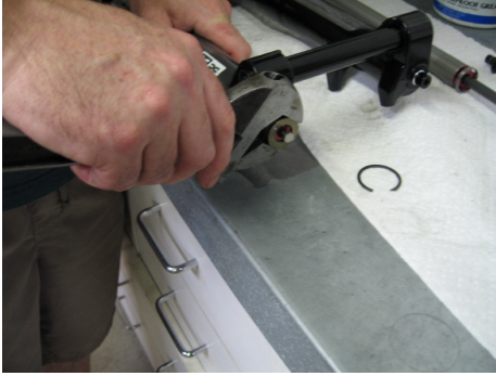
For 35 mm Boxxer Team/World Cup remove rebound base bolt adjuster
