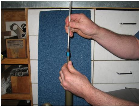
Cycle rod to remove any air bubbles and insert the rebound adjust rod
