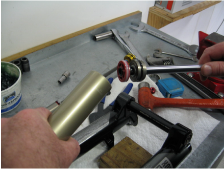
For 35 mm Boxxer Race rebound damper rod assembly shown removed
