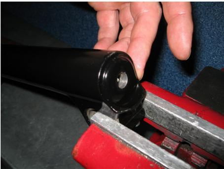
Deburr the hole and remove any visible chips
