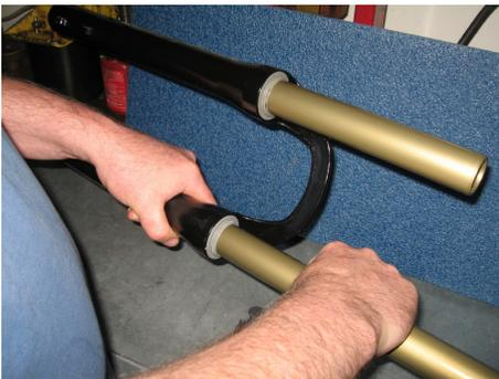
Push the slider tube all the way in until it contacts the bottom of the leg
