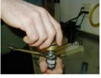
Screw on fork cap, make sure the cartridge rods bottoms on cap and bring jam nut up to contact cap
