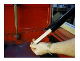
Using a spring to apply pressue to the cartridge tube air impact the base valve from the lower lug.
