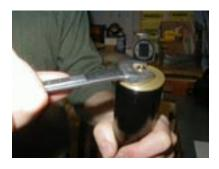
Tighten jam nut to fork cap, do not over tighten because this will damage the rod. Snug the fork cap to the upper leg hand tight.
