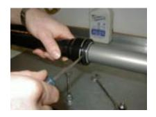
Remove clip. Heating the upper tube around the seal area with a propane tourch will ease the seal and bushing removal.
