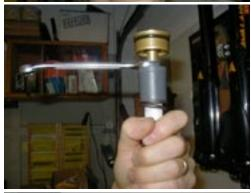
Using a 15 mm wrench loosen the fork cap from the cartridge rod by squeezing the wrenches together.
