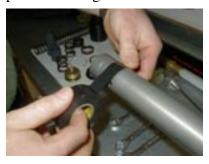
Apply a thin film of grease to the dust seal and oil seal
