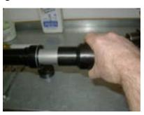
Install clip, be sure that it is seated in groove, press on dust seal.
