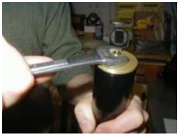
Inset the 14 mm wrench to keep the spring from moving.
