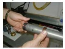
Using a 37 mm seal driver, install bushings and seal.
