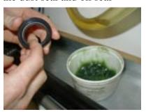
Install dust seal, clip, oil seal, washer, bushing. and slider.
