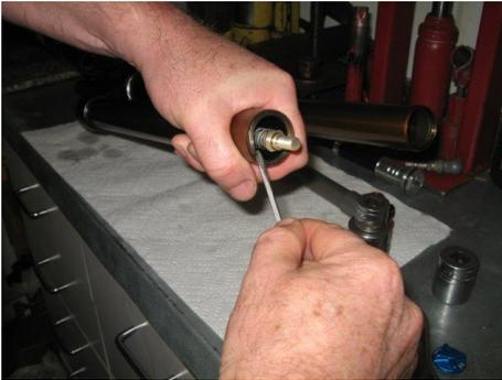
On the damper stanchion check for a snap ring groove at the bottom, some stanchions do not have the groove and the oil lock ring cannot be used with this fork and cartridge. Not to worry the hydraulic anti-bottoming system is secondary as compared to the air spring ramp-up created by the air side and is not required for most fork set-ups. Keep the oil lock ring and snap ring in a safe place as if the upper stanchions are ever replaced they most likely could be use on these new stanchions.
