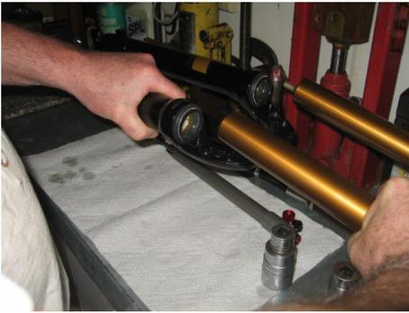
Gently separate the upper sliders from the lower casting
