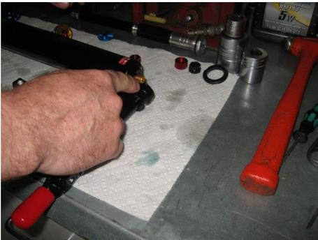
Thread the factory nut onto the shaft
