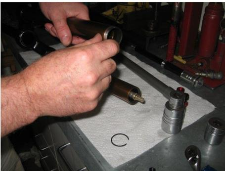
Install the abs oil lock ring, with the I.D. chamfer facing out.
