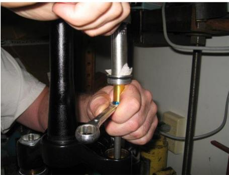
Using a 1/2 inch wrench and 15mm 6 point socket tighten the jam nut. **Be very careful these parts are delicate. Use a paper towel on the fork cap hex to avoid scratching the finish.**
