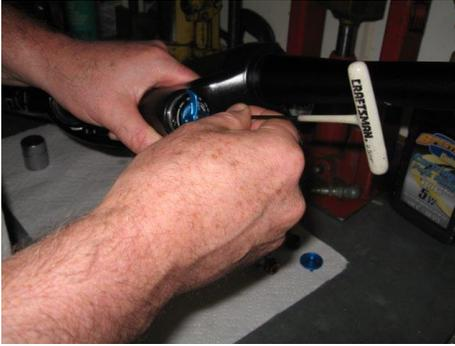
Using a 2mm Allen wrench loosen remove the bolt retaining the compression knob
