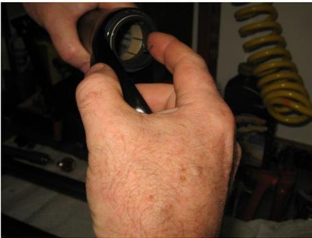
Apply new grease to the dust seal
