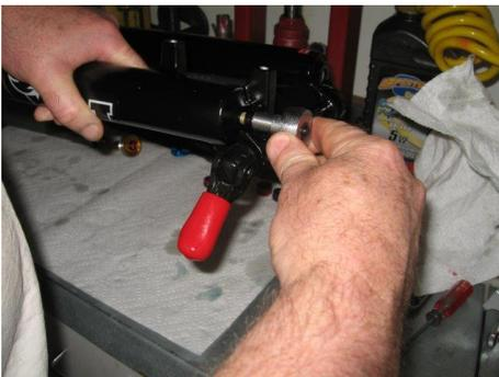
Tighten the nut snug, do not try to torque as it will just crush the washer
