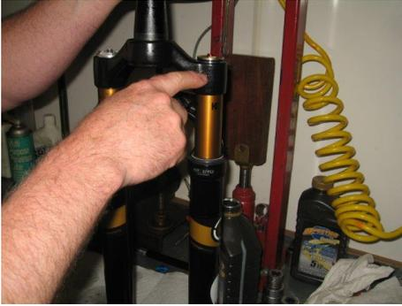
Thread the fork cap in by hand initially
