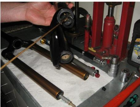
Remove the bottom out bumper you will not need this, only on the damper side, the air side bumper can remain installed to prevent damage to the stanchions from severe bottom out.
