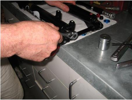
Using a 10mm Ratchet loosening the retaining nut on the spring leg
