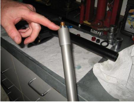
Apply a bit of grease to the 1.5 x 12 mm o-ring on the ABS cone of the Avalanche Cartridge
