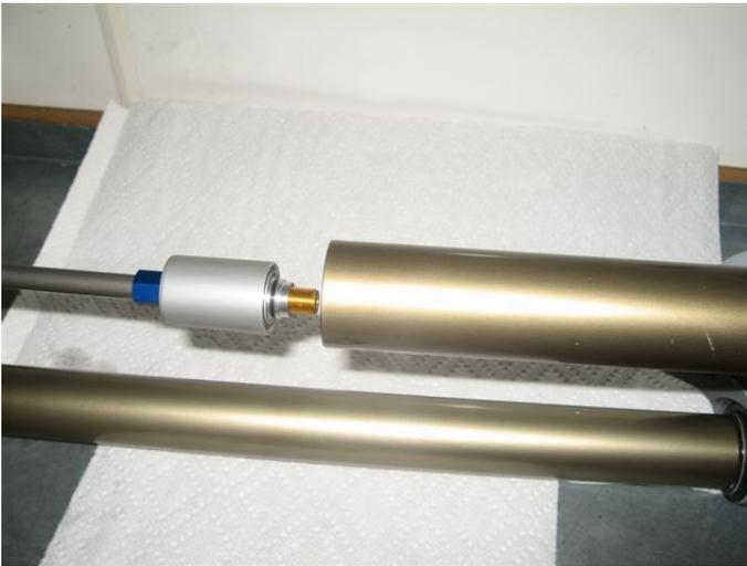
Remove the cartridge damper assembly.
