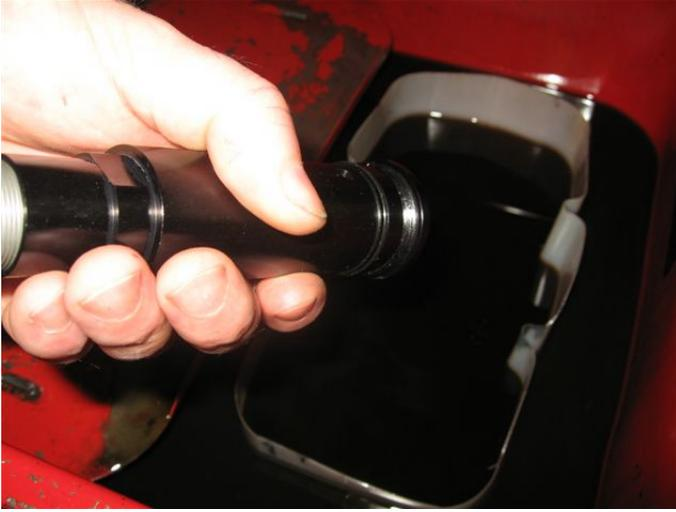
Dump and cycle rod to remove oil from damper.
