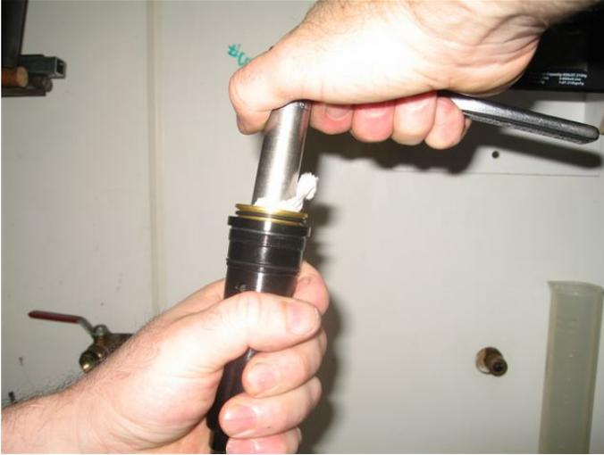
Tighten the inner cap with a 6 point 15 mm socket.
