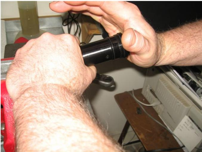
With the cartridge outer chamber wrench flats clamped gently in the vise, plunge the inner chamber fork cap assembly into the outer chamber and rotate clockwise to start the fork cap threads, turn as many turns as possible by hand.
