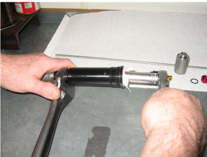
Using a wide adjustable wrench and a 6 point 15 mm socket loosen the inner fork chamber cap assembly.
