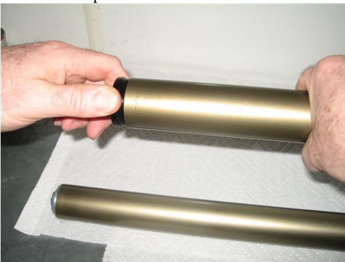
Thread the outer fork cap into the stanchion, being carefull not to cross thread.
