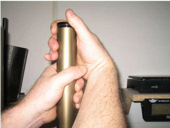
Hand tighten the outer fork cap.
