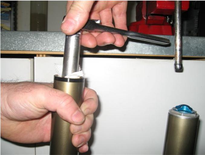
The cap must not be tightened with the wrench, only hand tight.
