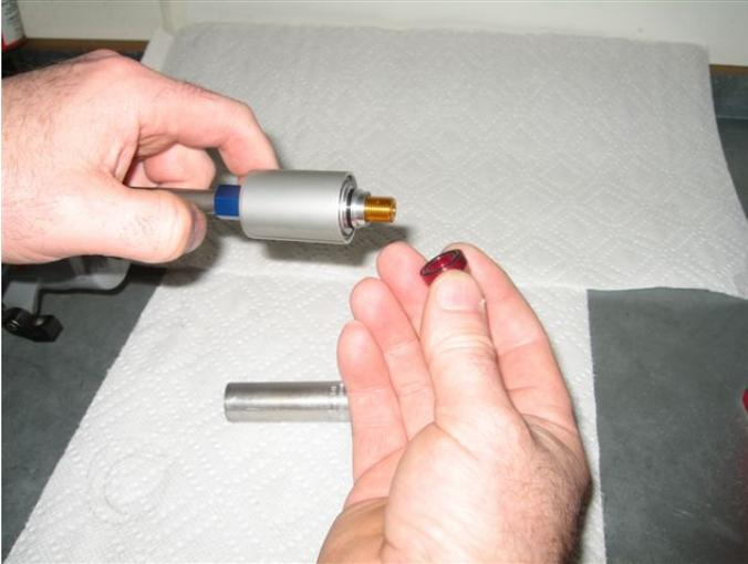
Remove the red nut and o-ring.
