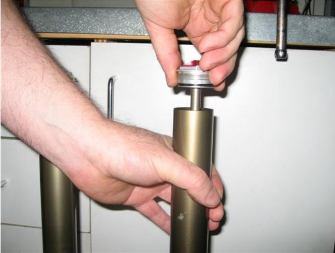
Unscrew fork cap and dump any oil that might of leaked from the damper, out the stanchion.
