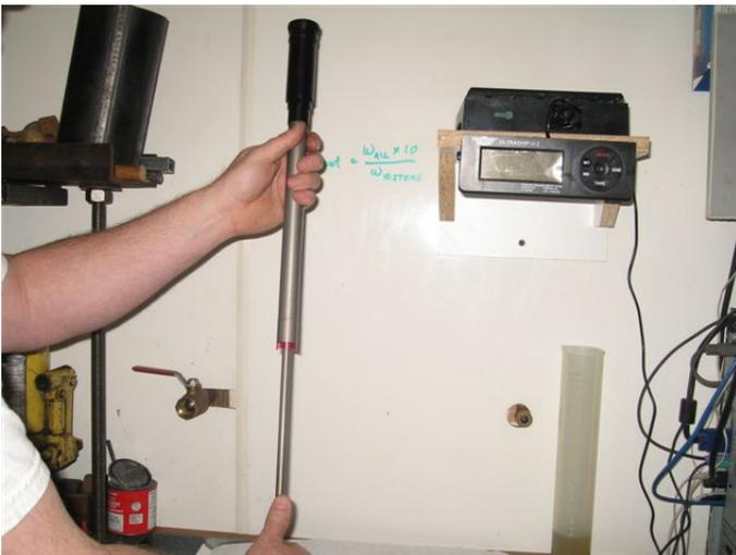
Using very short strokes at first, starting at 1 in compression strokes, then 2 inch and so forth until all 8 inches of stroke is completely bled, bleed the air
