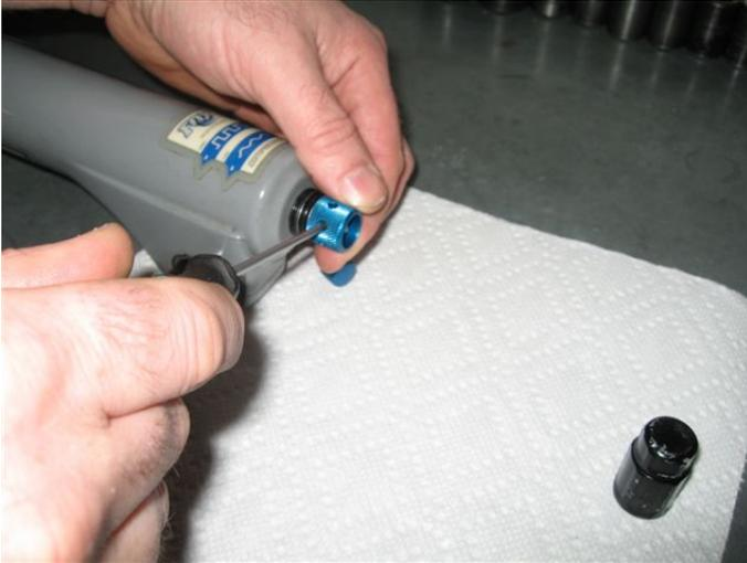
With an Allen key, remove the high speed knob.
