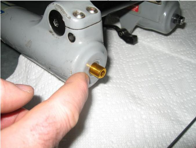
Make sure you can see the abs cone starting to protrude into the lower leg hole.
