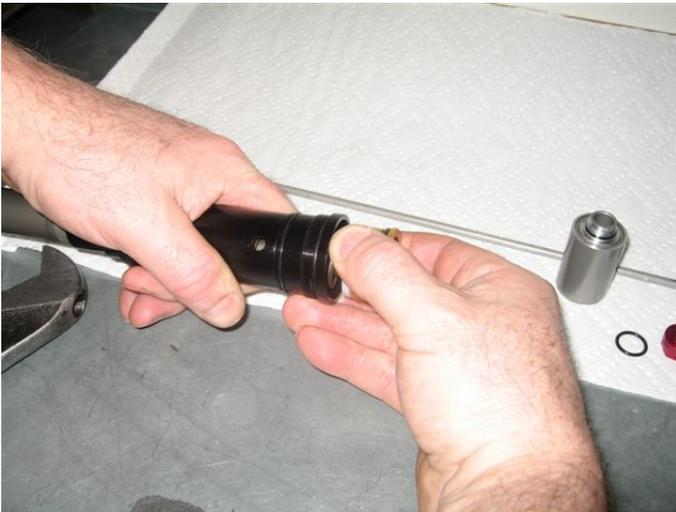
Remove the inner chamber cap assembly.
