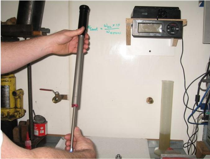
Make one final stroke and dump any excess out of the outer chamber cap holes. The damper should be clear of air bubbles and no hissing sounds should be heard when cycling the damper rod.
