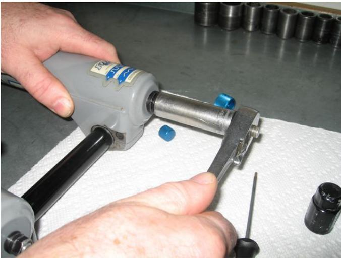
Remove base bolt adjuster nut.
