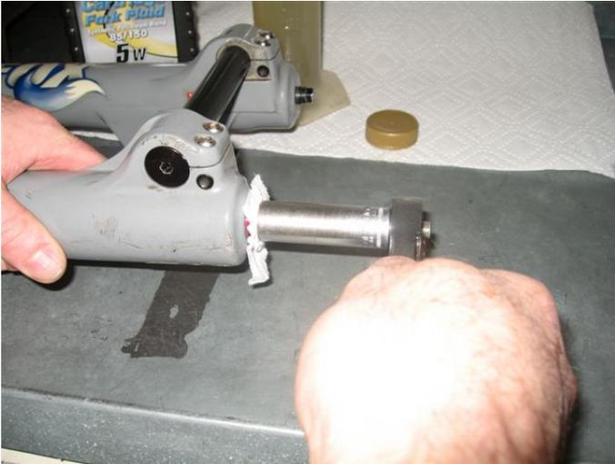
Tighten the lower adaptor nut to 15-20 inch-lbs.
