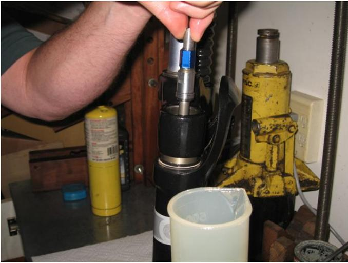
Cycle cartridge rod up and down completely until smooth consistent damping with no air bubbles.
