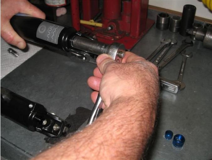
Loosen base nit with 15 mm socket.
