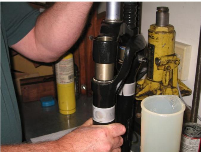
Cycle upper stanchion to remove air bubbles between casting and stanchions.
