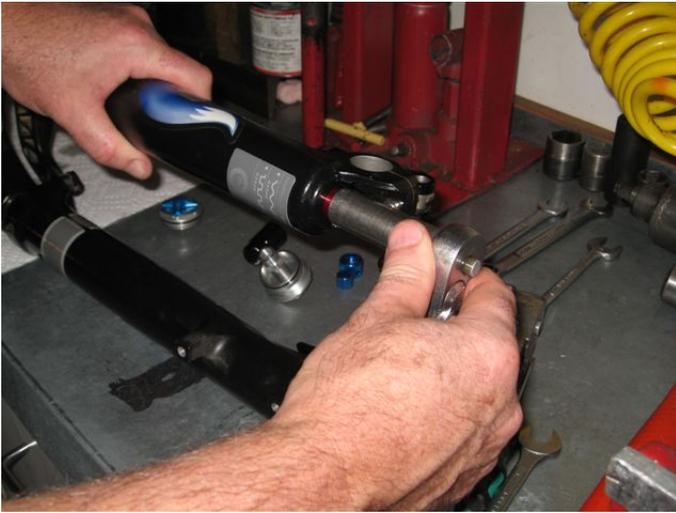
Snug up adaptor nut and tighten to 15-20 inch-lbs.
