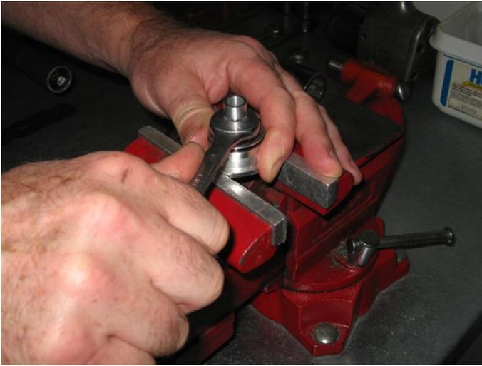
torque, after bottoming tighten 1/16 turn.
