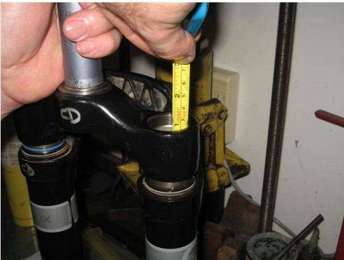
For 2006-14 models, adjust oil height to 30 mm(1.18 inches) from top with all components fully compressed. For 2015-17 models, adjust oil height to 40 mm(1.57 inches) from top with all components fully compressed.
