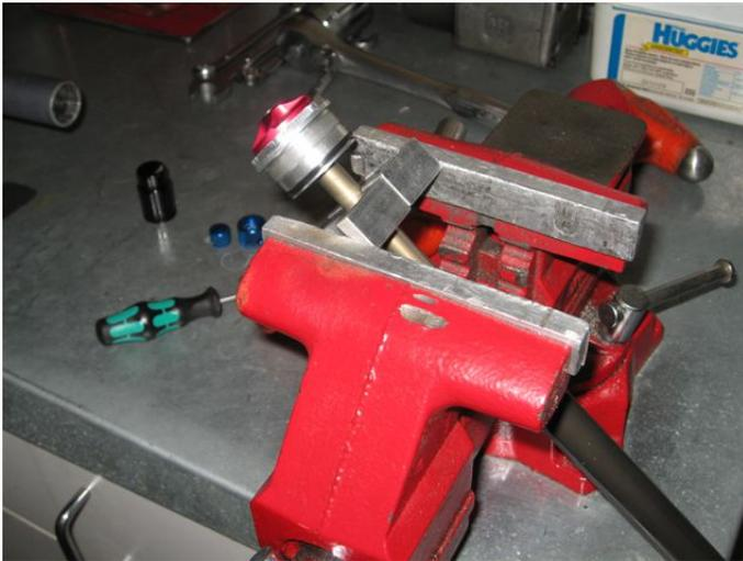
Remove stock fork cap for 2016-2014 models. Clamp the cartridge rod with 10 mm shaft clamps. 2015-17 models skip to installing cartridge in stanchion.
