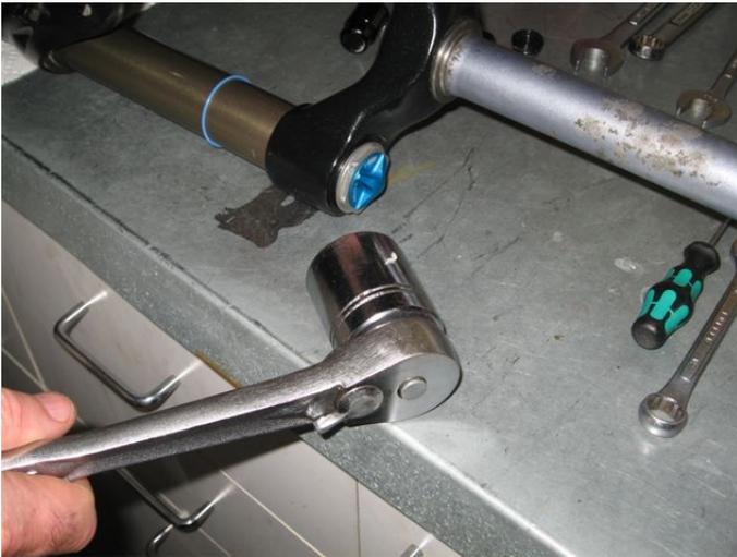
Remove fork spring/air cap to allow forks to be compressed. **Warning: If it is an air fork be sure all pressure is released before removing cap assy.**
