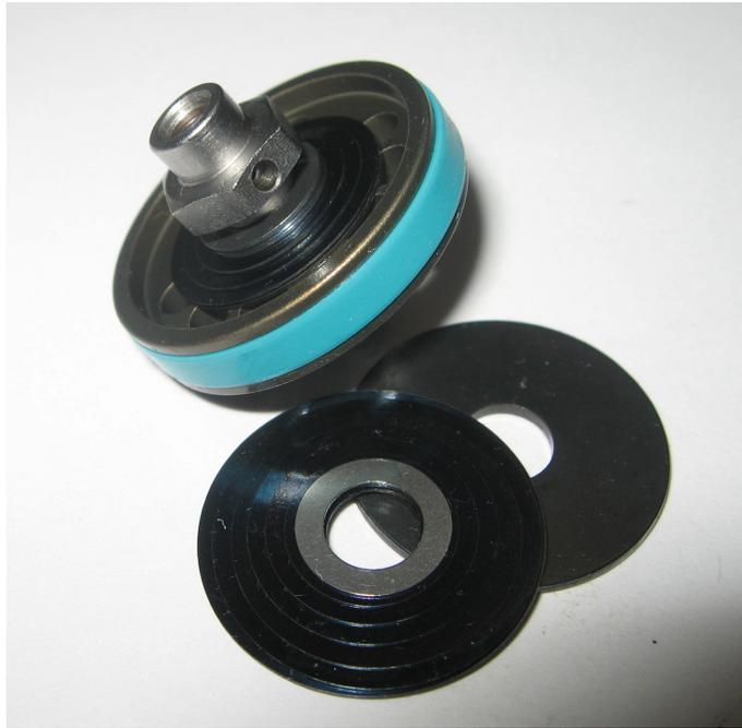
The removal of the Propedal and replacement with the SSD compression adjuster system now allows the main piston to be revalved for speed sensitive valving shims according to the linkage progression, rider ability and type of terrain.
