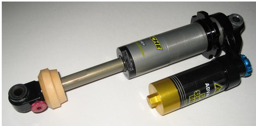
DHX 5.0/4.0 with Extended Reservoir and Shape Factor Bottom-out Bumper
