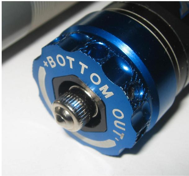
The nitrogen chamber bottom-out adjuster on the the DHX 5.0
