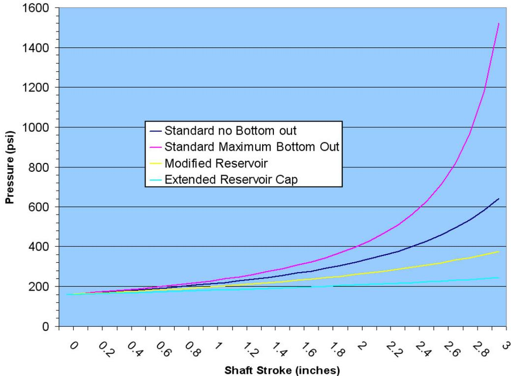
**For a 1/2 inch diameter shaft, 1500 psi equals 294 lbs extra spring force in other words for a 300 lb/in spring at 3 inches of stroke, the spring rate would increase to 400 lb/in.**
