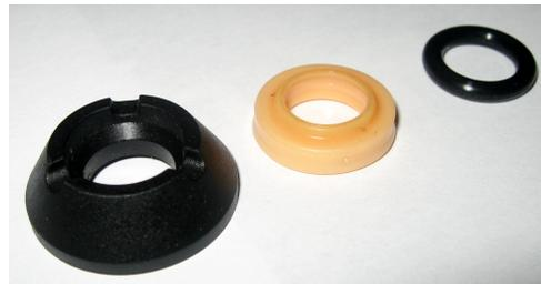
Stock DHX Bumper, Dust Seal and Oil Seal
