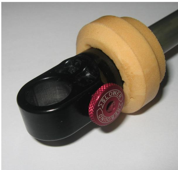
Once your sag is set properly the rebound adjuster can be set for the ride conditions, standard position is about 7 clicks counterclockwise out from full slow. Turn out 1 click to speed up rebound, this will make it absorb small close together bumps easier. Turn in 1 click to slow up rebound when absorbing big bumps to prevent kicking up. Repeat click at a time until desired results are achieved. Faster rebound is more desirable when trying to achieve plusher setting
