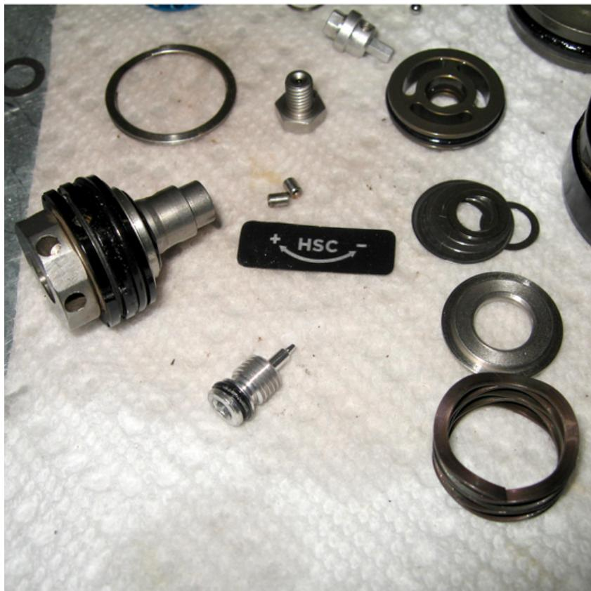
*Disassemble High/Low speed adjuster*
