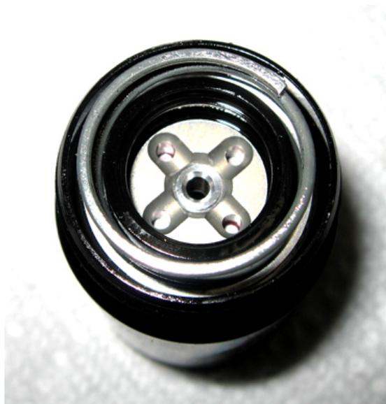
*SSD valve installed in place of Boost valve*
