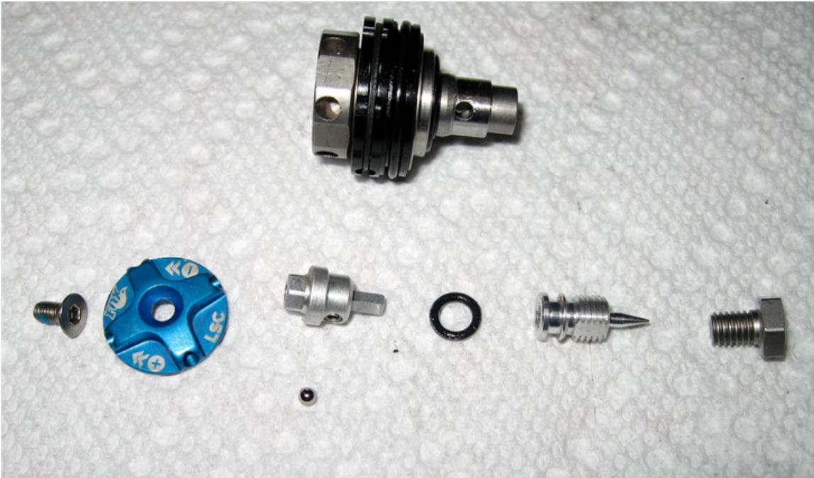
*Low Speed Adjuster exploded view
