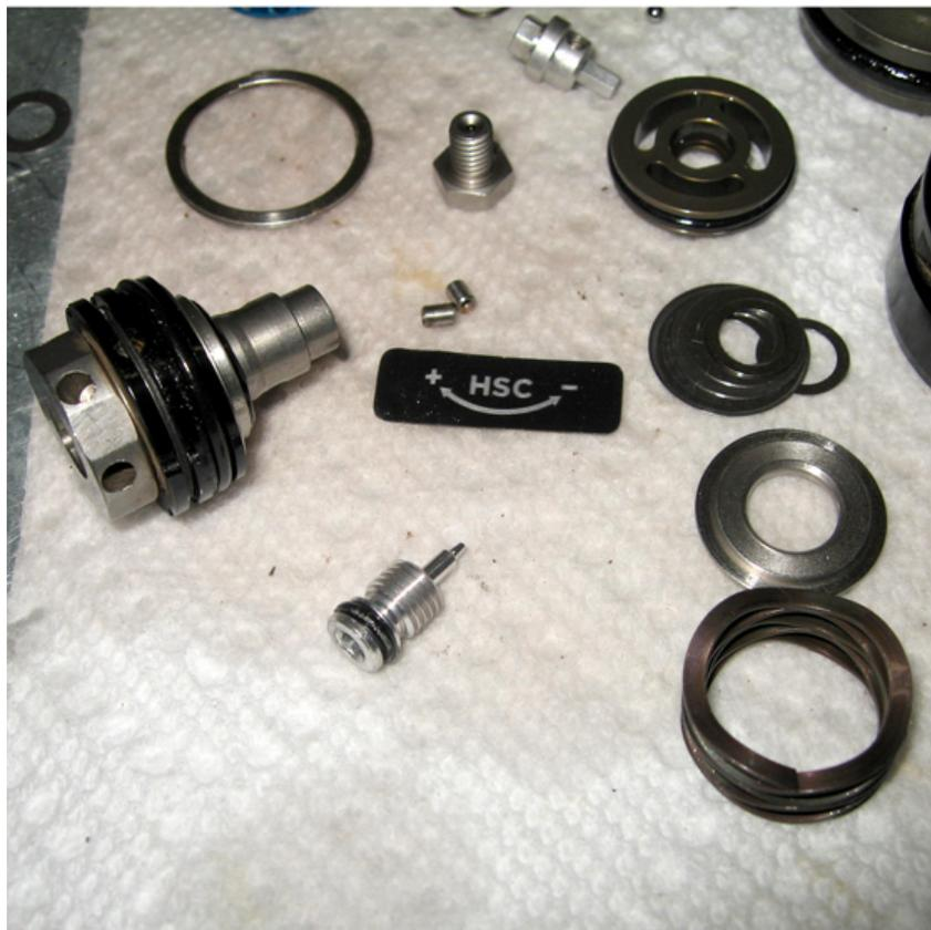
*Disassemble High/Low speed adjuster*
