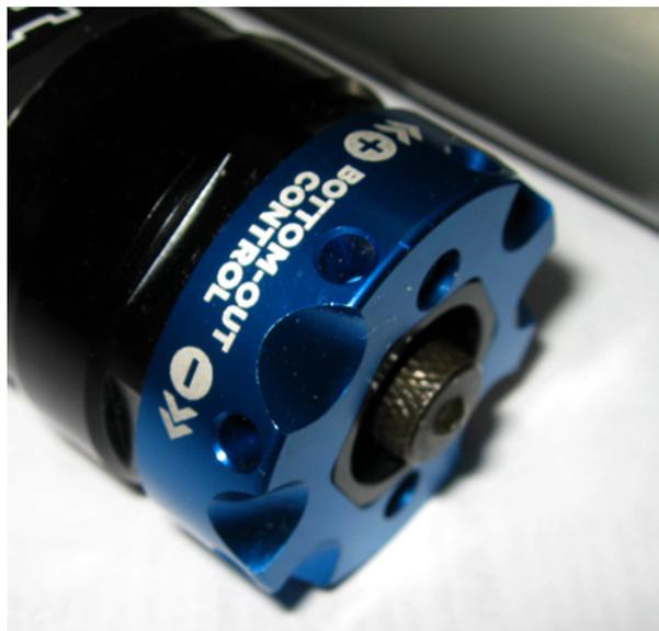
The nitrogen chamber bottom-out control on the the RC4
