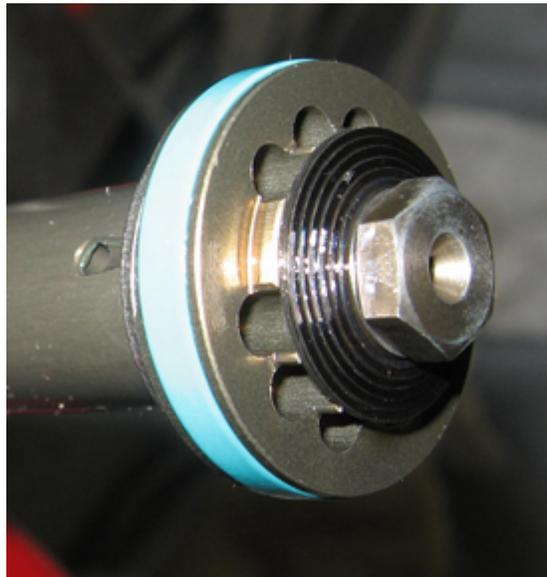
***Main Piston shown with revalved shims installed***
