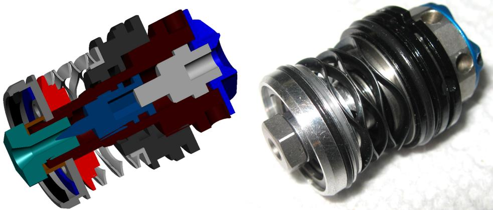
*Low Speed Plunger and High Speed Valve*
