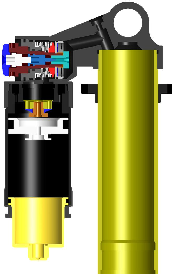
*Transition Adjuster and SSD valve shown installed*
