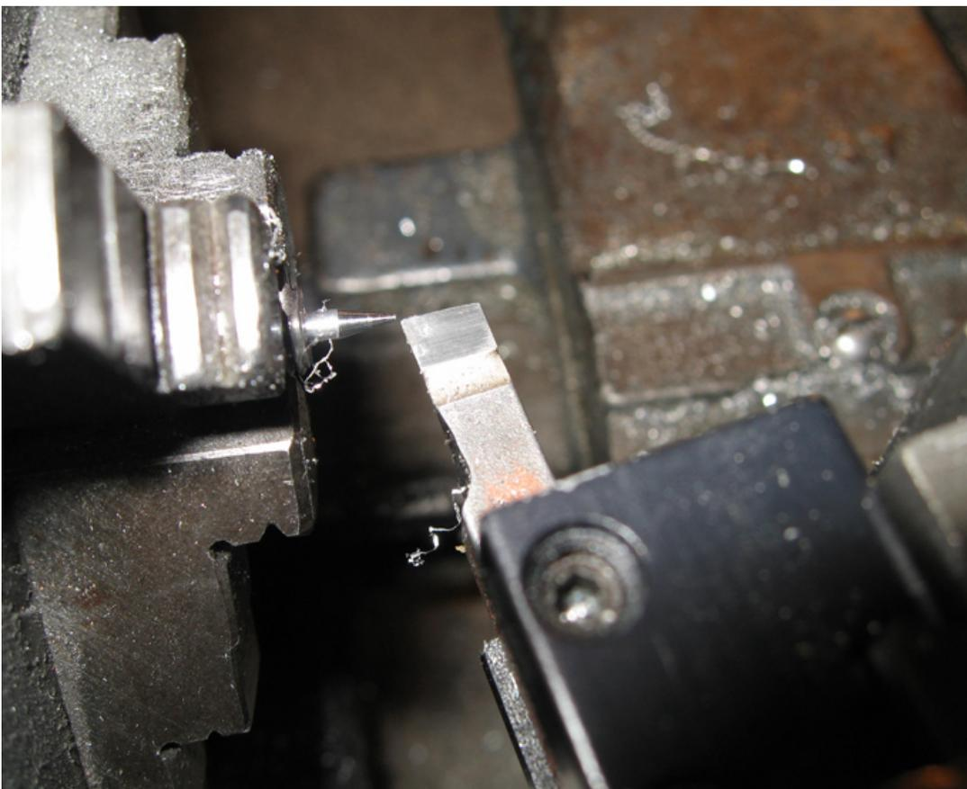
*Change needle taper for wider adjustment range*
