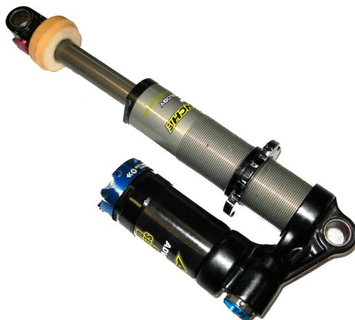
Fox RC4 with SSD, Transition and Shape Factor Bottom-out Bumper upgrade.
