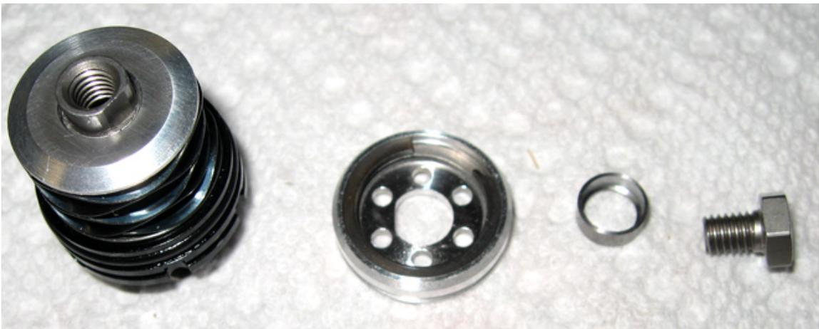
*High/Low Transition valve exploded view
