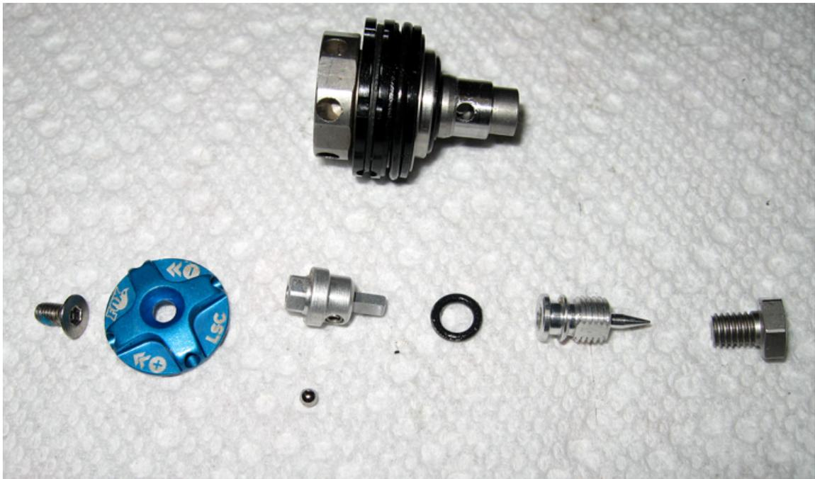
*Low Speed Adjuster exploded view
