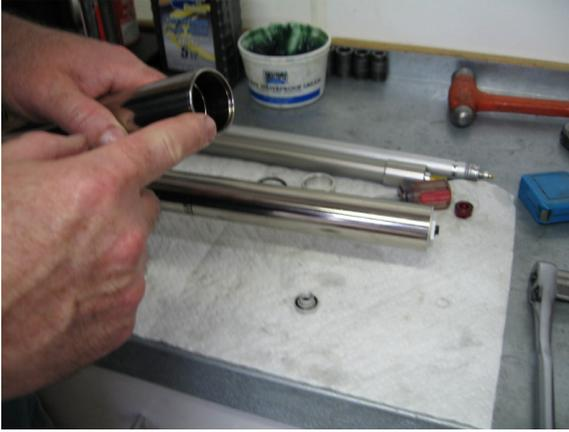
Locate and inspect the lower grooves in the stanchion.
