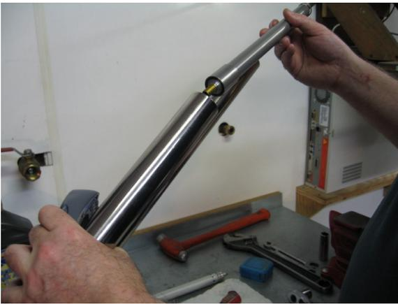
Install the cartridge in the lowers, be sure the the o-ring provided does not fall off, you can use grease or rvtv to help secure it.
