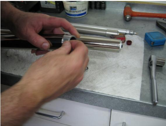
Install the oil lock ring with the inside chamfer facing out/down, look for an arrow or blue dots to depict the chamfered end. The EVO tapered stanchion requires 2 snap rings, install the first in the upper groove, then the oil lock ring with chamfer facing down and the lower snap ring.
